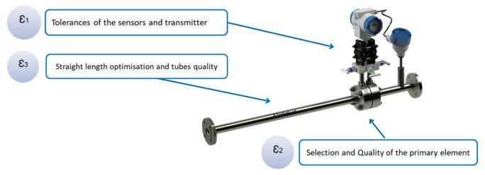
Control of all the components of this measurement device, in accordance with the standards requirements, selection of reliable and high-quality products, close manufacturing control during assembly in order to offer a device intended to achieve a high accuracy measurement around 0,5%.
